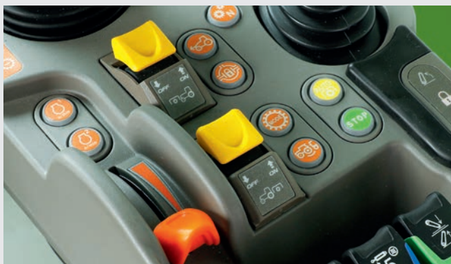
↑ Easy engagement of front and rear PTO through buttons on MaxCom armrest.
