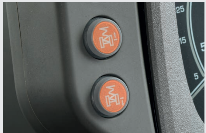
↑ Two new dedicated buttons allowing manual adjustments of the position of the front suspension.
